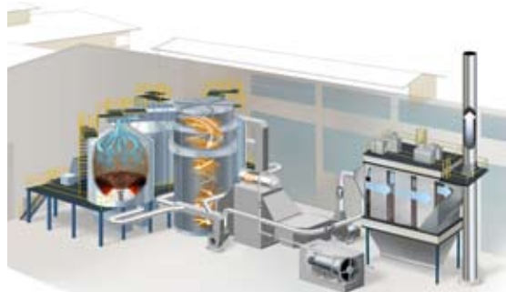
Figure 2: Configuration of 20 MWt/1.4 MWe CHP plant
