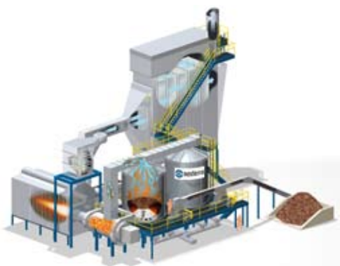
Figure 3: Configuration of 12 MWt Direct Fired Boiler System
